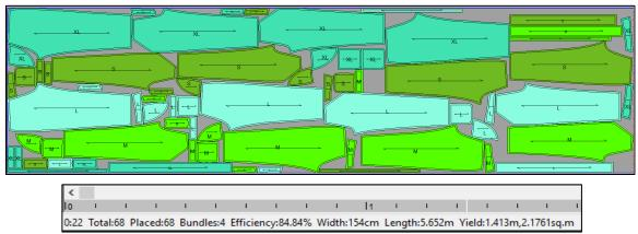
Figure 5 Illustrative example of a centre to selvedge colour-shading marker
