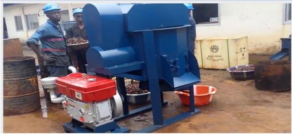
Figure 4.40: Improved version of fabricated processing mill designed by FINIC in Freetown
