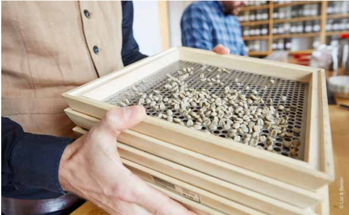
Screens for grading bean size.
