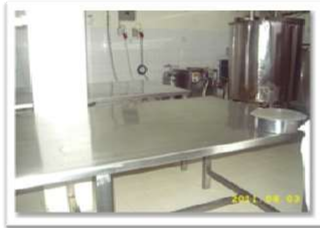
Figure 23: Smooth and inert work surfaces facilitate cleaning and help avoid build-up of food.
