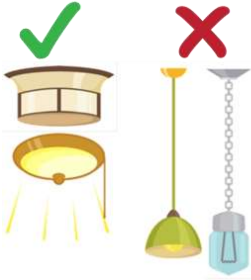
Figure 36: Protected lighting fixtures can prevent contamination from breakages.
