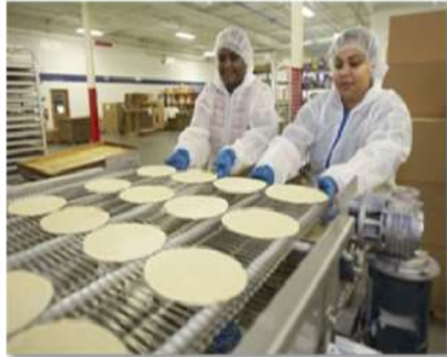
Figure 30: Removable grill allows for cleaning below and in-between surfaces.
