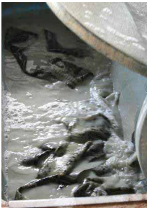
Figure 25 Processing of skins to “wet blue” stage (Viet Nam)
