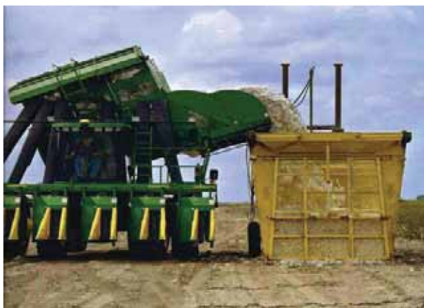
Figure 2.4: Spindle picker dumping into a module builder
