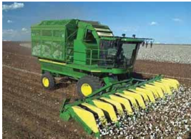
Figure 2.2: Typical stripper harvester for cotton
