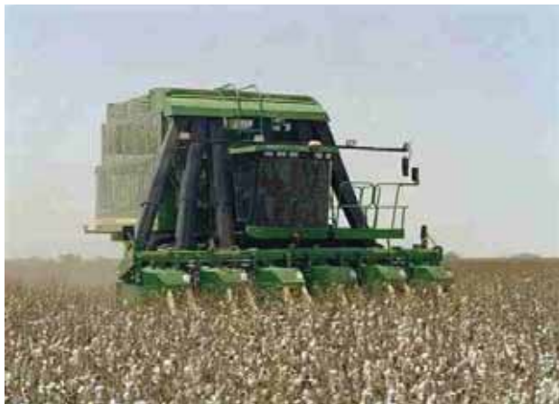
Figure 2.1: Typical spindle-type mechanical harvester for cotton
