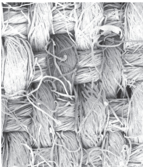
Figure 2.42: Woven fabric (plain weave pattern)
