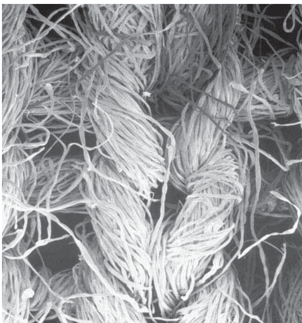
Figure 2.46: SEM of knitted fabric
