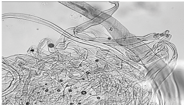
Figure 2.18: White speck nep (highly magnified) attached to mature fibre
